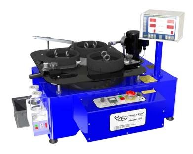
The Lapmaster Model 15 lapping / polishing machine is fitted with an electronic dispenser for the liquid diamond abrasive slurry and the appropriate lubricating fluid, a dual head spray bar and an electrically driven stirrer unit which houses small glass reservoirs of both fluids
